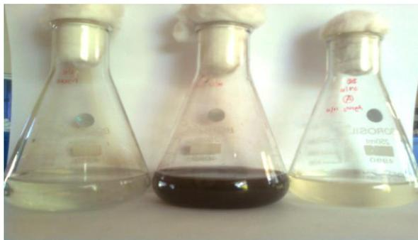
**Fig.2** Nitrate reductase positive results using in the extra cellular filtrate of the silver nanoparticles synthesized by *Streptomyces* sp
