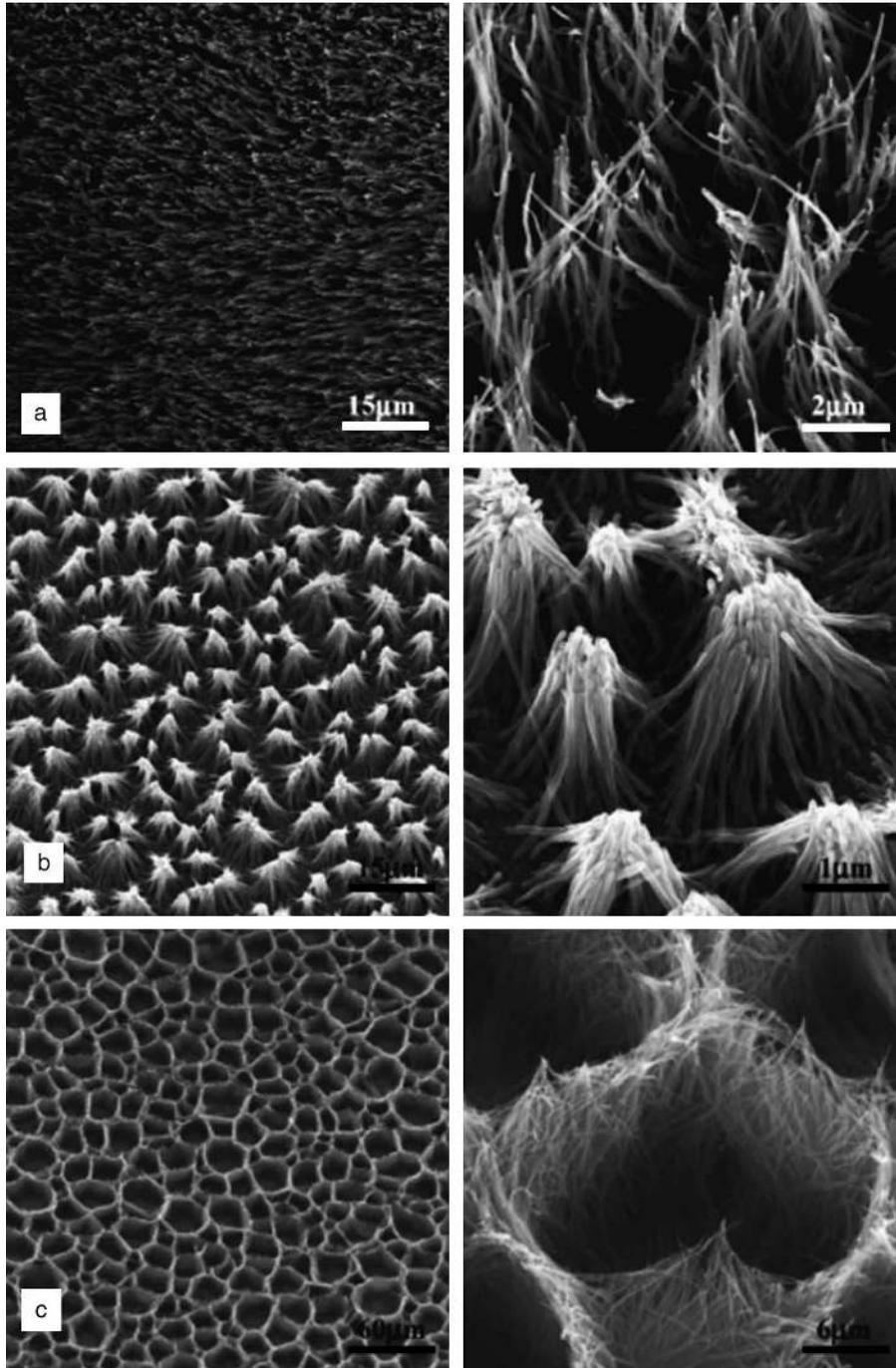
Figure 11. Examination by SEM of the MWCNTs-based structures. (a) Perpendicular aligned carbon nanotubes; (b) Pyramid-like structures which are formed after a physicochemical treatment; (c) Network of cross-linked carbon nanotube walls forming cavities. Reprinted with permission from (Correa-Duarte et al. 2004). Copyright (2007) American Chemical Society.
