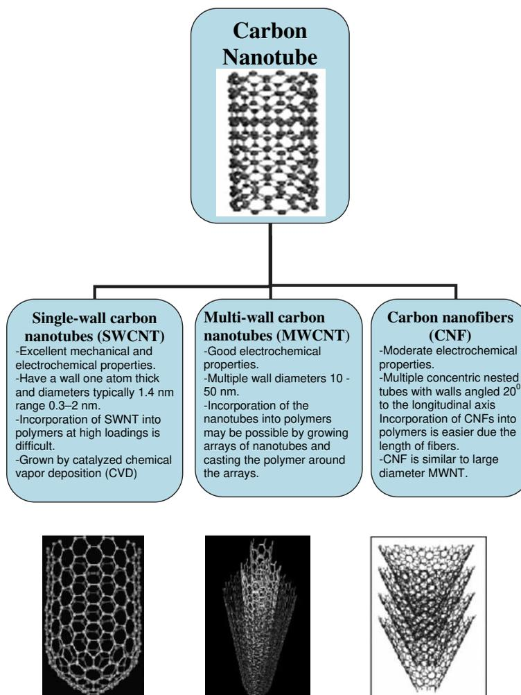
Figure 1. Various forms of carbon nanotubes and their general properties (Kang et al. 2006).
